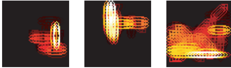
Figure 2.3: Example visualizations of prototypes taken from Serre et al. [1], corresponding to airplanes (left), faces (middle), and motorcycles (right). Here, an oval indicates the location and scale of an edge detector (i.e., an S1 unit), while color indicates the contrast of those edges.
